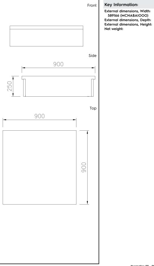
Modular Cooking Range Line thermaline 90 - 900 mm Closed Work top, 1 Side
